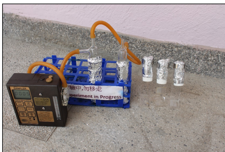
Fig. 4. Calibrating of the diffusion rate of the passive sampler by impinges with a constant flow pump.
