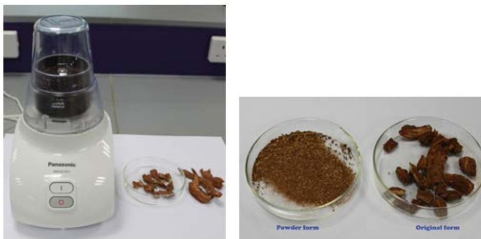
Fig. 2. A blender is used to breakdown the solid sample into powder.
