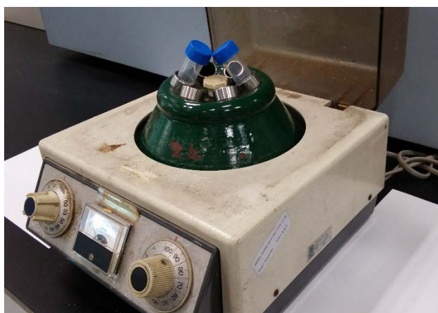
Fig. 2. Centrifuge tubes are placed diagonally so that mass is well-balanced.
