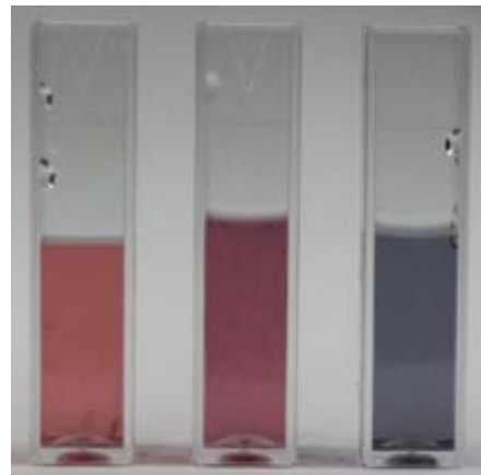
Fig. 4. AuNPs testing solution (left); milk sample mixed with AuNPs without melamine (middle); milk sample mixed with AuNPs in the presence of 10 ppm melamine (right).
