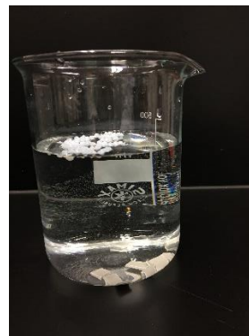
Figure 10. Separation/Isolation of PS from the mixture.
