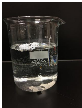
Figure 9. Addition of sodium chloride solution to plastic mixture.
