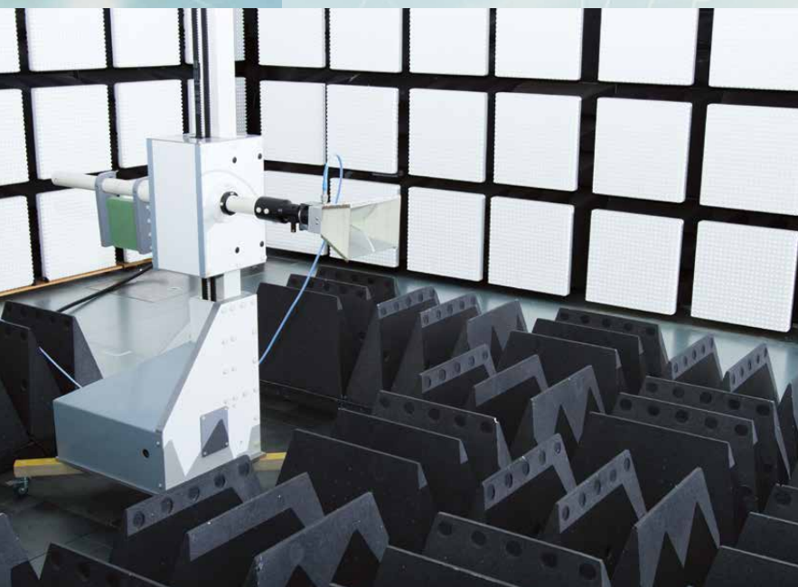
EMC tests ensure electrical devices will not interfere with the operation of other devices in its vicinity
