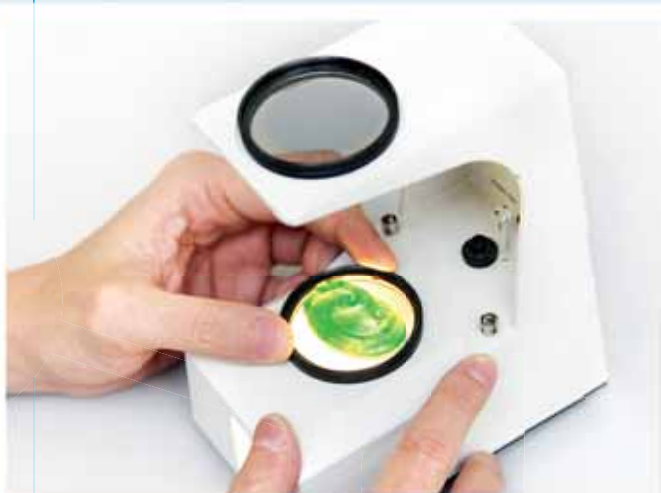
Analysis of Fei Cui using Polariscope
