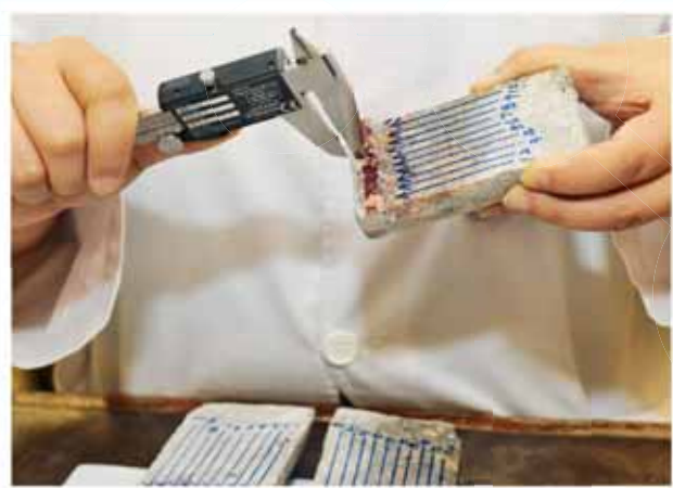
Measurement of carbonation depth in concrete sample
