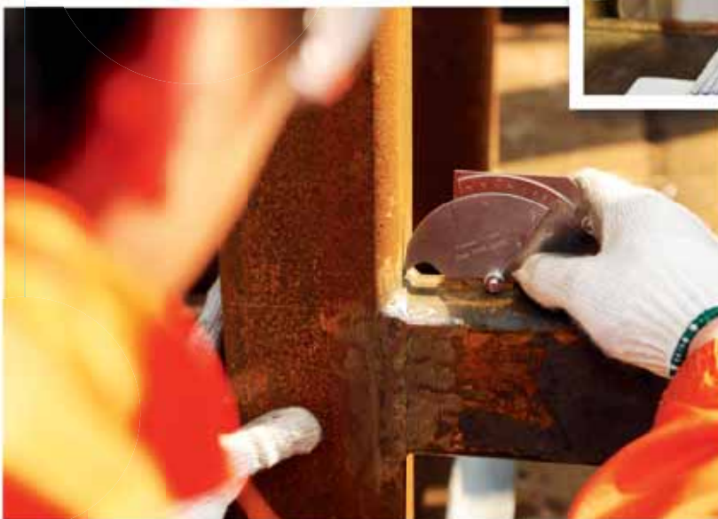
Thickness measurement of weld using weld gauge
