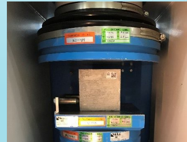
Carrying out compression test within the required testing time frame
