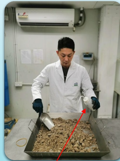
Adding water and mixing
