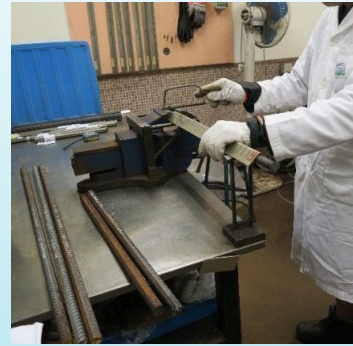
Inscribing equidistant marks on test specimen
