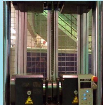
Tensile test (removing extensometer upon yielding)
