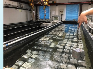
Manually placing test samples into curing tank
