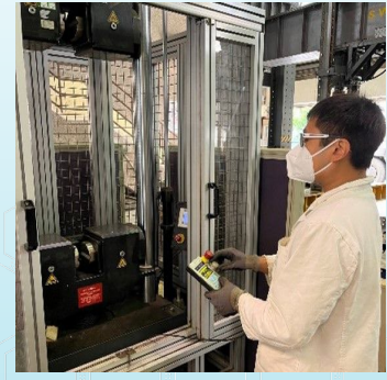
Setting up Universal Testing Machine
