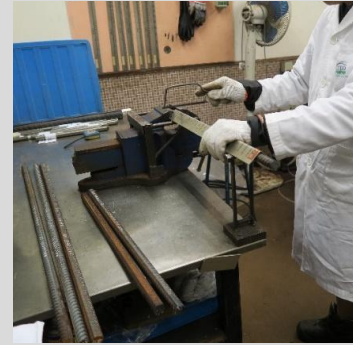
Inscribing equidistant marks on test specimen
