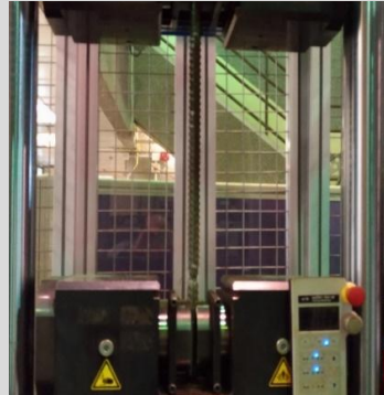
Tensile test (removing extensometer upon yielding)
