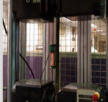
Fixing extensometer to the test specimen
