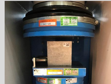
Carrying out compression test within the required testing time frame
